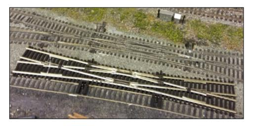
"A major task to be tackled in July is the replacement of the double slip at Woodside. After nearly 30 years it is becoming life-expired and unreliable. The main difficulty is the restricted access under the layout here as at least one point machine has to be moved".
